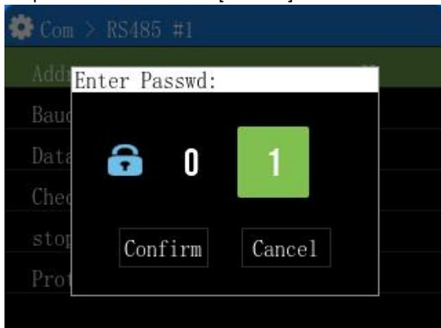
5、 Press the key “←” to enter the [Addr] selection page, enter the address in the input box, and click [Confirm] to set the device address
